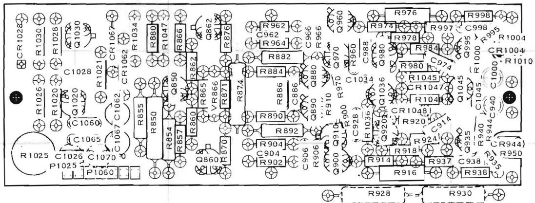
Fig. 8-5. A3—Fast Rise Board component locations.
