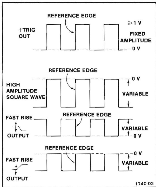
Fig. 2-3. Output signals from the PG 506 Calibration Generator.
