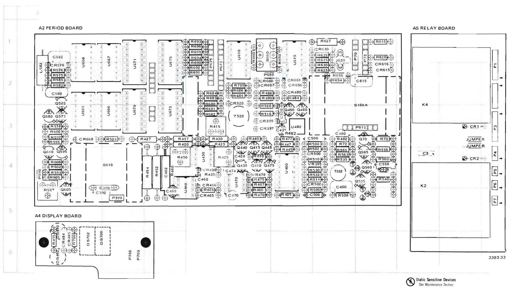
Fig. 8-4. A2—Period and A4—Display Board component locations.
