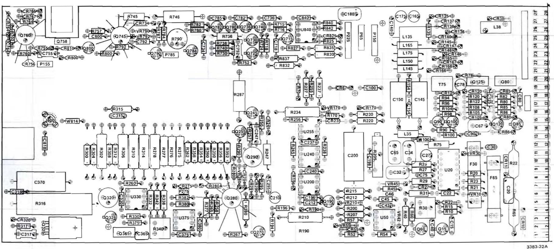
Fig. 8-3. A1—Main Board component locations.
