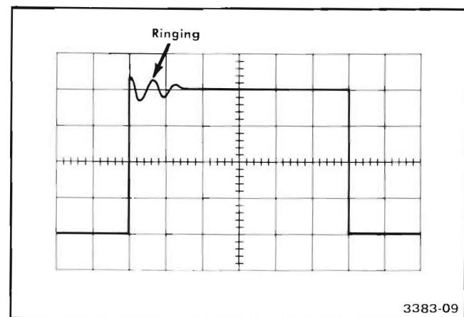
Fig. 2-8. Typical waveform showing ringing at front corner.
